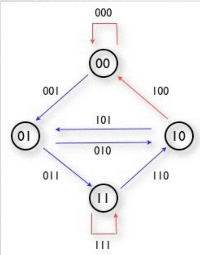
$$M_0 = \begin{matrix} & \begin{matrix} 00 & 01 & 10 & 11 \end{matrix} \\ \begin{matrix} 00 \\ 01 \\ 10 \\ 11 \end{matrix} & \left( \begin{array}{cccc} \{ "000" \} & \emptyset & - & - \\ - & - & \emptyset & \emptyset \\ \{ "100" \} & \emptyset & - & - \\ - & - & \emptyset & \{ "111" \} \end{array} \right) \end{matrix}$$
